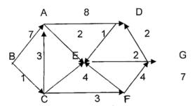
Find the shortest distance between B and G applying Dijkstra's Algorithm.
